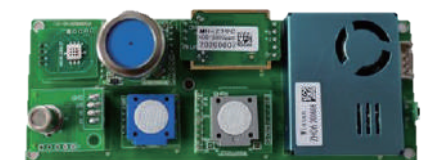
ZPHS01B 9-in-1 Air Quality Detection Module (CO2, PM2.5/10, TVOC, CO, O3, CH2O, NO2, T&H)
